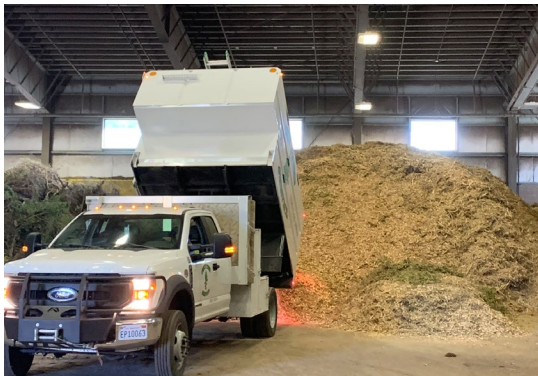
Figure 1: Waste woody material is currently collected, processed, and stored at STR until it is transported to Nevada for disposal. Material is sourced from defensible space thinning and C&D waste.
